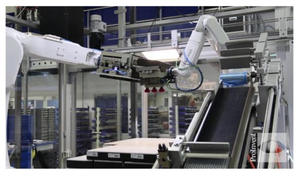
ProInvent has developed a system of vision guided, clean room robots, performing challenging inspection tasks with 3D coordinated movements. The process is performing with an OEE of 98% and ready for scaling.
